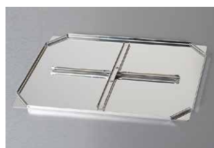
Platform for four microplates (Cat. No. 48010)
